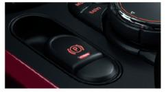
In place of the bulky brake lever, just press a button to activate the new Electric Parking brake. Leaving more room for comfort and a plush armrest.
