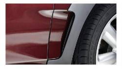
The new MINI Clubman is the first in the family to have these. Air is taken in from the front and channelled around the wheel arches to reduce turbulence before escaping through the side panels.
